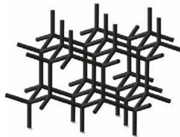
A portion of the diamond structure
