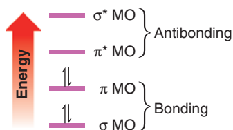
The relative energies of electrons involved in \sigma and \pi bonds.
