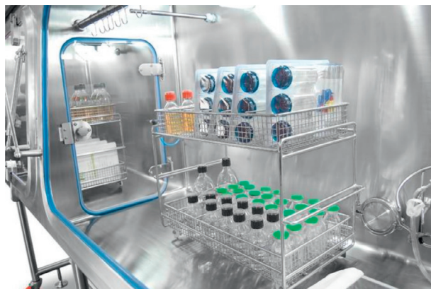
Figure 12.2 Isolator prepared for sterility testing. Photograph courtesy of Pharmig.
