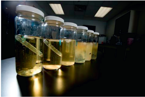
Figure 12.1 Biological indicators used to determine the sterility assurance level of an autoclave. Photograph: Tim Sandle.
