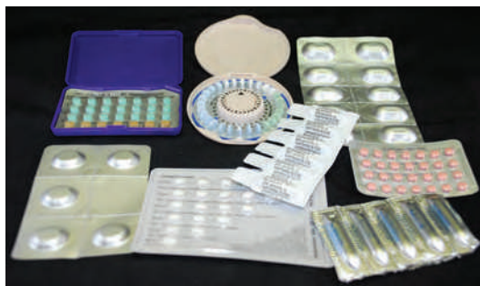
FIGURE 3.6 Commercial blister packaging of pharmaceuticals.
