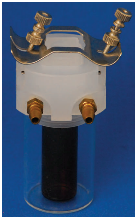
FIGURE 11.3 A microdiffusion cell for working with very low quantities of drugs and solutions.
