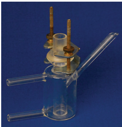
FIGURE 11.2 Typical Franz diffusion cell. The donor cell is on top, and the upper and lower chambers are separated by either a membrane or skin. A solution or semisolid containing the drug is placed in the upper cell and a receiver solution in the lower cell. The angle tube on the right is for sampling and fluid replacement. The two ports on the left consist of an inlet and outlet where constant temperature water can be circulated.
