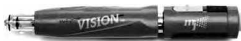
FIGURE 15.28 Medi-Jector II, a jet injection device. The jet injection method uses pressure rather than a needle to provide subcutaneous distribution of medication. This device can be used with U-100 insulin or a combination of insulins and can deliver 2 to 100 units in half-unit increments. (Courtesy of Antares Pharm Inc.)
