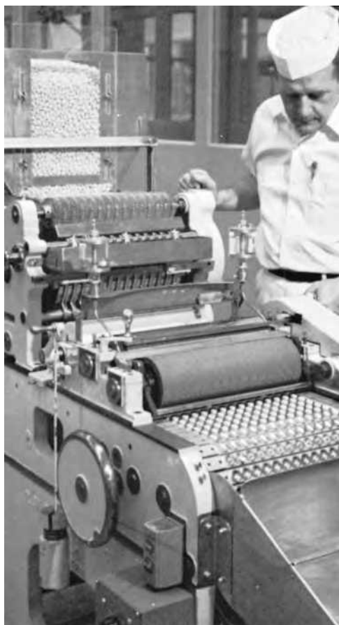
FIGURE 8.33 Branding of coated compression tablets on a Hartnett branding machine. (Courtesy of Pfizer, Inc.)
