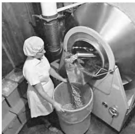
FIGURE 7.15 Cleaning and polishing hard-filled capsules using the Accela-Cota apparatus. (Courtesy of Eli Lilly and Company.)
