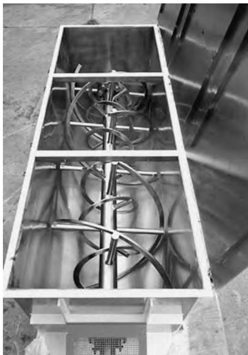
FIGURE 6.3 Ribbon blender used for mixing powders and preparing granulations. (Courtesy of Littleford Day.)
