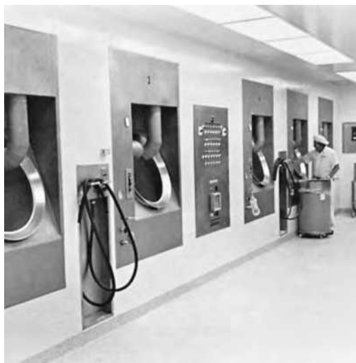
FIGURE 8.31 Modern tablet-coating facility. Air and exhaust ducts to assist drying are automatically operated from central board. (Courtesy of Eli Lilly and Company.)
