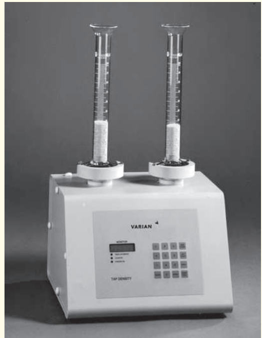
Tapped density tester (Courtesy of Varian Inc.)
