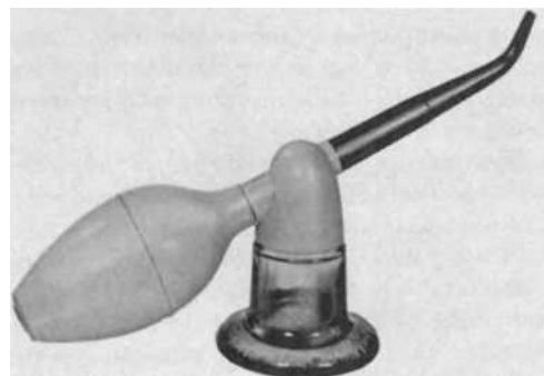
FIGURE 6.8 A general-purpose powder blower or insufflator. The powder is placed in the vessel. When the rubber bulb is depressed, internal turbulence disperses the powder and forces it from the orifice. Powders may be delivered to various body locations such as the nose, throat, tooth sockets, or skin. (Courtesy of DeVilbiss Company.)
