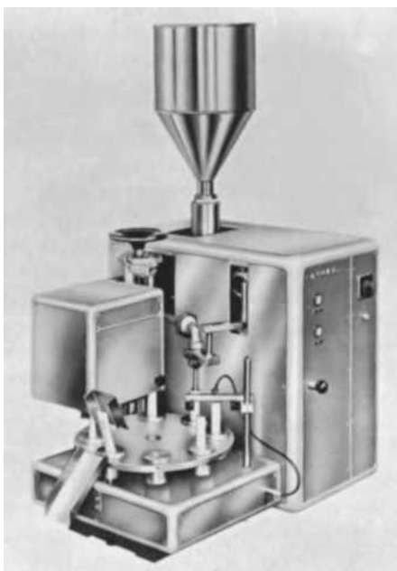
FIGURE 10.8 A small-scale fully automatic filling and crimping machine for collapsible metal tubes. The capacity of the machine is up to 60 units per minute. (Courtesy of Chemical and Pharmaceutical Industry Co.)
