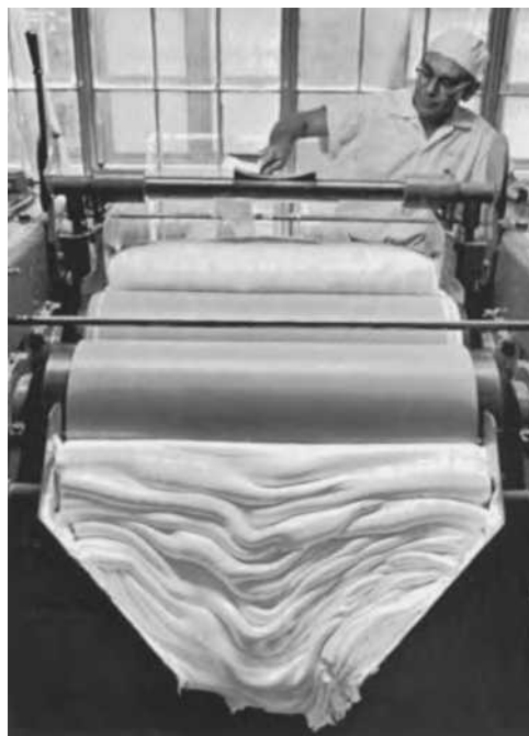
FIGURE 10.5 Day ointment roller mill. Standards of fineness and smoothness require that no grains of material be visible under a 10-power microscope after passage through this machine. (Courtesy of Eli Lilly and Company.)
