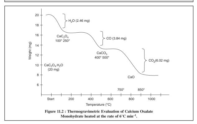
**Stage 1 :** The water of hydration (or crystallization) from calcium oxalate monohydrate is lost which corresponds to 2.46 mg (12.3%) equivalent to 1 mole of  $H_2O$  in the temperature range 100-250°C.
