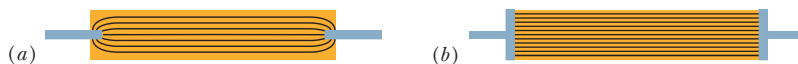
Figure 26-8 Two ways of applying a potential difference to a conducting rod. The gray connectors are assumed to have negligible resistance. When they are arranged as in (a) in a small region at each rod end, the measured resistance is larger than when they are arranged as in (b) to cover the entire rod end.
