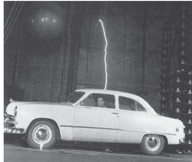
Figure 24-22 A large spark jumps to a car's body and then exits by moving across the insulating left front tire (note the flash there), leaving the person inside unharmed.
