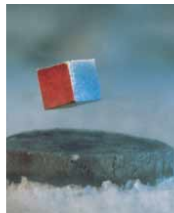
A small permanent magnet levitated above a disk of the superconductor \text{YBa}_2\text{Cu}_3\text{O}_7 , which is at 77 K.
