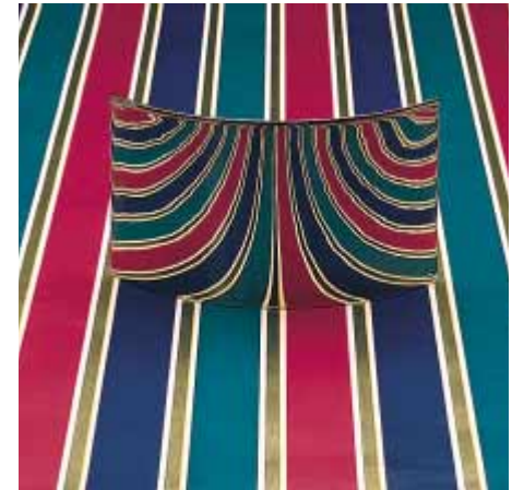
Reflection of parallel lines from a convex cylindrical mirror. The image is virtual, upright, and reduced in size.
