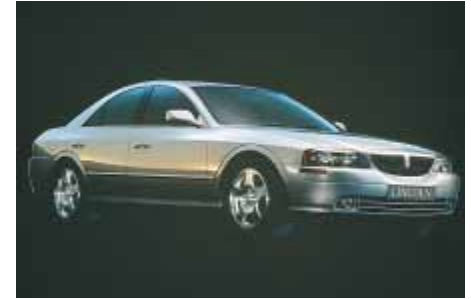
Aerodynamic car. A streamlined body reduces air drag and increases fuel efficiency.
