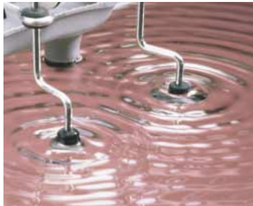
Interference of water waves produced in a ripple tank. The sources of the waves are two objects that oscillate perpendicular to the surface of the tank.
