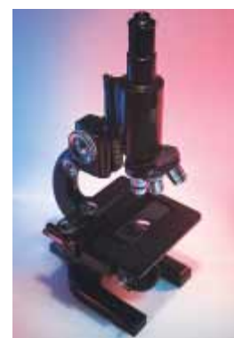
Figure 36.41 (a) Diagram of a compound microscope, which consists of an objective lens and an eyepiece lens. (b) A compound microscope. The three-objective turret allows the user to choose from several powers of magnification. Combinations of eyepieces with different focal lengths and different objectives can produce a wide range of magnifications.
