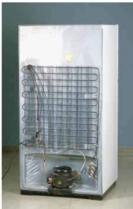
Figure 22.14 The coils on the back of a refrigerator transfer energy by heat to the air. The second law of thermodynamics states that this amount of energy must be greater than the amount of energy removed from the contents of the refrigerator (or from the air in the kitchen, if the refrigerator door is left open).
