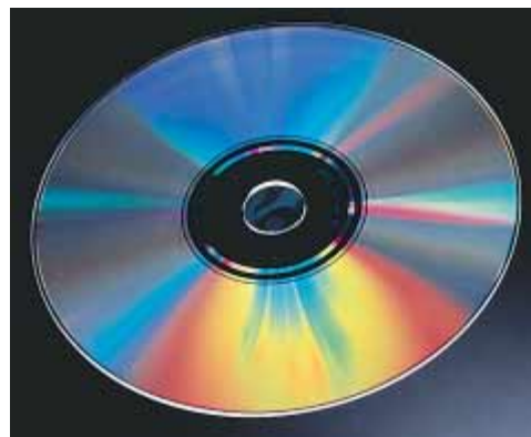
Figure 38.22 A compact disc observed under white light. The colors observed in the reflected light and their intensities depend on the orientation of the disc relative to the eye and relative to the light source.
