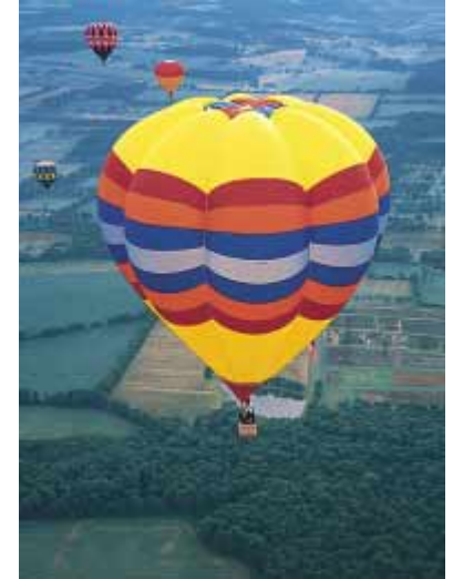
Hot-air balloons. Because hot air is less dense than cold air, a net upward force acts on the balloons.
