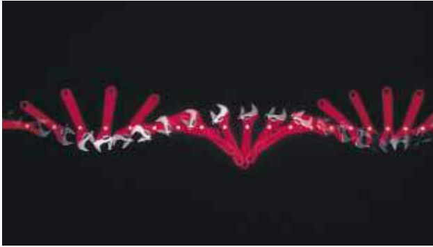
Figure 9.25 Multiframe photograph showing an overhead view of a wrench moving on a horizontal surface. The center of mass of the wrench moves in a straight line as the wrench rotates about this point, shown by the white dots.
