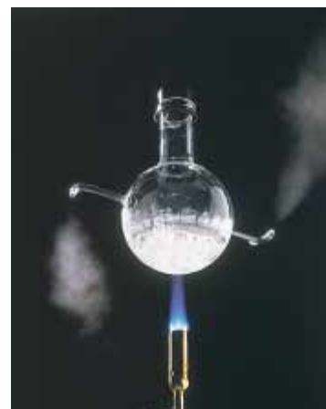
This device, called Hero's engine , was invented around 150 B.C. by Hero in Alexandria. When water is boiled in the flask, which is suspended by a cord, steam exits through two tubes at the sides (in opposite directions), creating a torque that rotates the flask.
