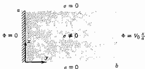
FIG. 7.12b Two-dimensional conductive solid embedded in a nonconductive medium.
