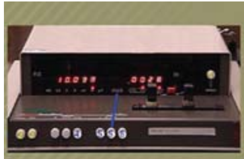
Capacitance Measurement using bridge
