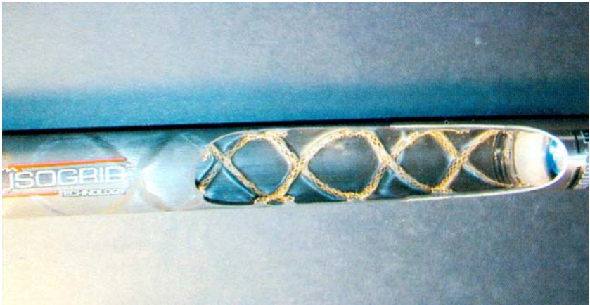
9.12 Cut-away view of an 'Isogrid' bicycle frame tube to show inner stitched fiber core reinforcement (courtesy Vyatek Corp.).
