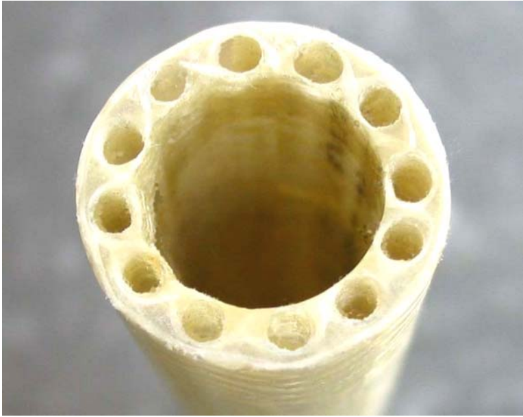
9.22 'Technical plant stem' with double-braid textile construction.
