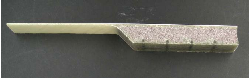
9.11 Increasing bending stiffness of composites using a foam core.
