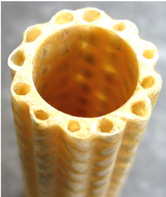
9.23 'Technical plant stem' with partial polyurethane foam matrix.
