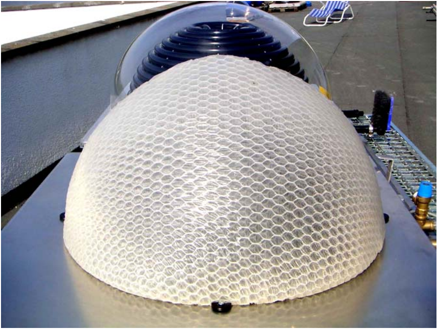
10.14 Deep-draw (formed with heat and pressure) spacer textile as collector cover.
