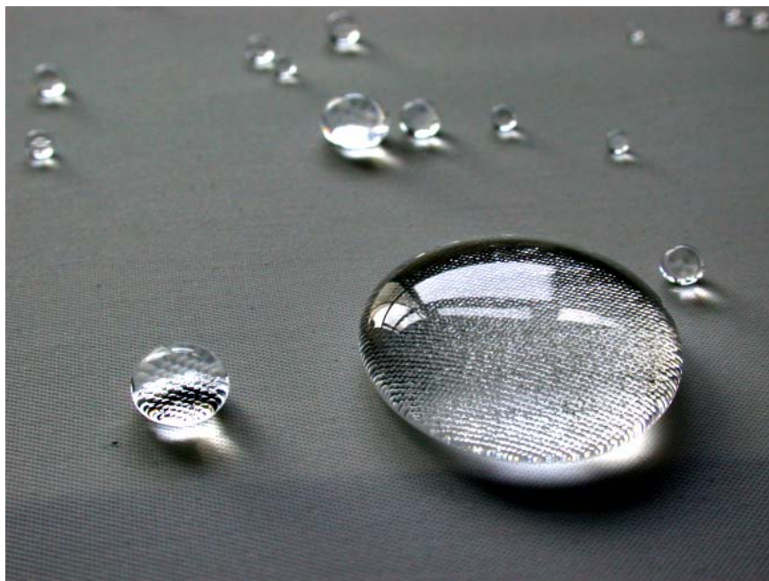
10.1 Spherical water drops on fabric with Lotus Effect.
