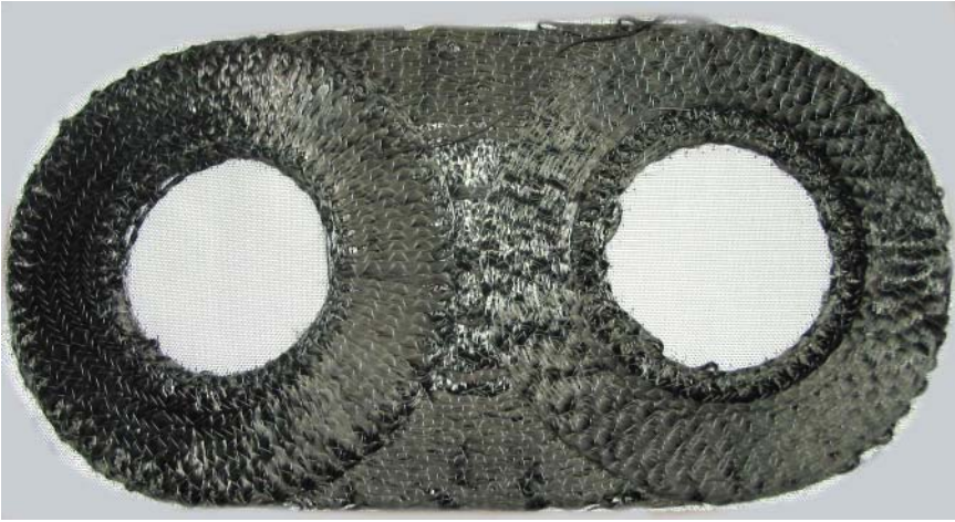
9.5 Example of a tailored fiber placement preform.
