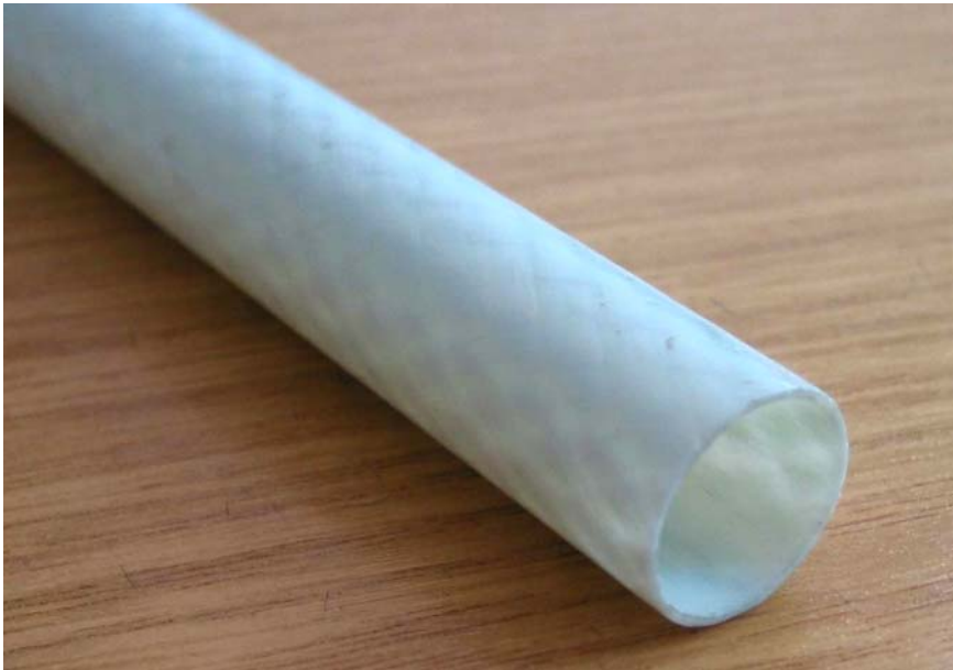
9.21 Braid-pultruded tubular profile with thermoset matrix.
