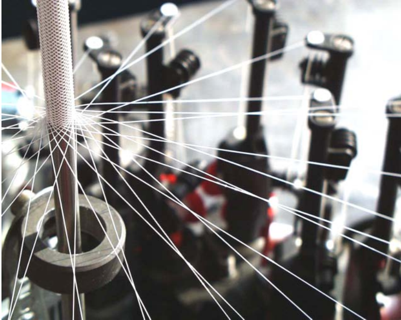
9.19 Detail of braiding technique.
