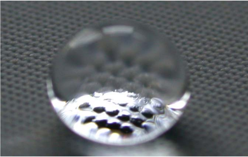
7.3 Water drop on superhydrophobic textile surface.
