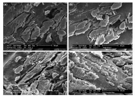
**Fig. 13-23** SEM images of PHB–plasticizer–flax systems: (a) PHB–flax, (b) PHB–GTA– flax, (c) PHB–TBC–flax, and (d) PHB–PEG–flax. (Reprinted from Wong et al., 2002, Properties of poly(3-hydroxybutyric acid) composites with flax fibers modified by plasticiser absorption, *Macromolecular Materials and Engineering* 287:647–655. Copyright Wiley-VCH Verlag GmbH & Co. KGaA. Reproduced with permission.)
