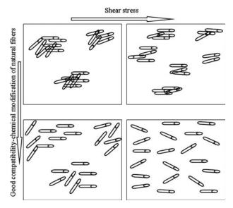
Fig. 11-6 Schematic of natural fiber mixing.
