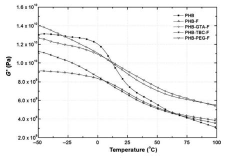
**Fig. 13-21** Storage moduli (G') of PHB and composites.
