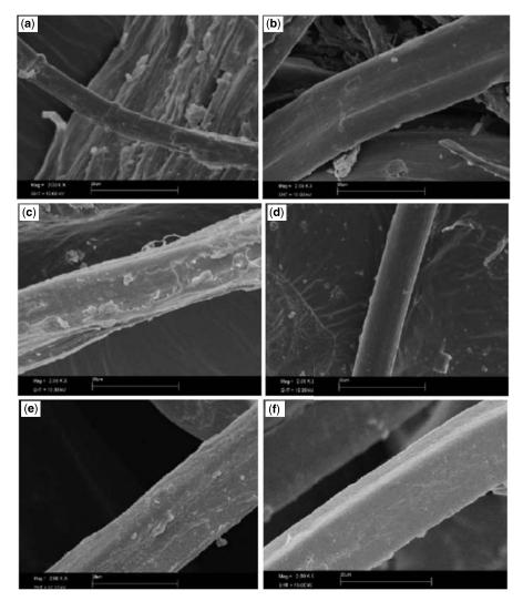
**Fig. 13-15** SEM images of untreated (a) and acetylated (b) flax fiber, untreated (c) and acetylated (d) hemp fiber and untreated (e) and acetylated (f) of wood fiber. (Reprinted from Tserki et al., 2005, A study of the effect of acetylation and propionylation surface treatments on natural fibers, *Composites Part A: Applied Science and Manufacturing* 36(8):1110–1118. Reproduced with permission from Elsevier.)
