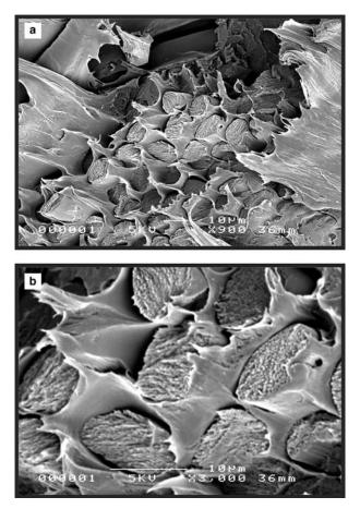
**Fig. 12-10** SEM images of the fractured surface of the original PLA/lyocell composites at different magnifications: (a)  $\times$  900, (b)  $\times$  3000.
