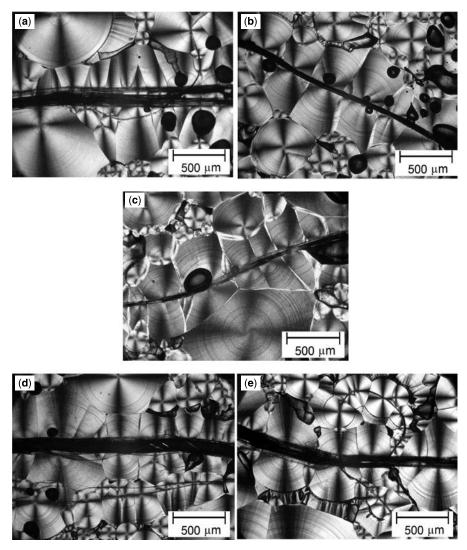
**Fig. 13-28** Optical micrographs of (a) unmodified PHB composite, and composites with (b) 2.5% TDP, (c) 5% TDP, (d) 7.5% TDP, and (e) 10% TDP. (Reprinted from Wong et al., 2004, Interfacial improvements in poly(3-hydroxybutyrate)–flax fiber composites with hydrogen bonding additives, *Composites Science and Technology* 64(9): 1321–1330. Reproduced with permission from Elsevier.)
