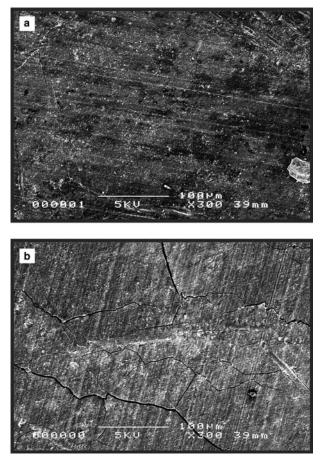
**Fig. 12-9** SEM images of the surface of the original and annealed PLA/lyocell composites: (a) original sample, and (b) annealed sample.
