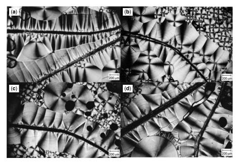
**Fig. 13-24** Optical micrographs of PHB–plasticiser–flax systems: (a) PHB–flax, (b) PHB– GTA-flax, (c) PHB–TBC–flax, and (d) PHB–PEG–flax. (Reprinted from Wong et al., 2002, Properties of poly(3-hydroxybutyric acid) composites with flax fibers modified by plasticiser absorption, *Macromolecular Materials and Engineering* 287:647–655. Copyright Wiley-VCH Verlag GmBH & Co. KGaA. Reproduced with permission.)
