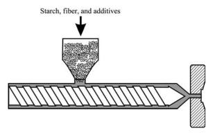
Fig. 14-5 A schematic representation of extrusion molding.
