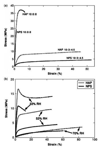
**Fig. 11-3** Stress-strain behavior of HAP (higher amylose-content potato starch) and NPS (normal potato thermoplastic starch) (10:3:4.5 and 10:0:8): (a) conditioned at 21°C and 53% RH; (b) at 33% RH, 53% RH, and 70% RH. (Reproduced with permission from *Biomacromolecules* **2006**, 7:981–986. Copyright 2008 American Chemical Society.)
