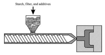
Fig. 14-3 A schematic representation of injection molding.
