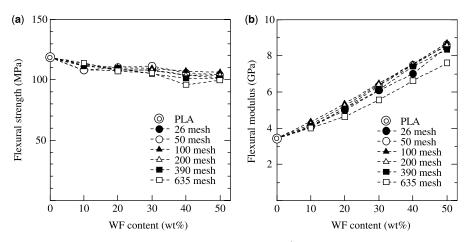
Fig. 12-5 Flexural properties of PLA/WF composites.
