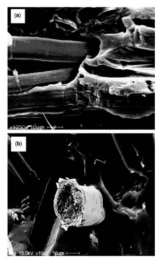
**Fig. 13-16** SEM images of fractured surfaces of (a) unmodified fiber composite and (b) acetylated fiber composite. (Reprinted from Zini et al., 2007, Biocomposite of bacterial poly(3-hydroxybutyrate-*co*-3-hydroxybutyrate) reinforced with vegetable fibers, *Composite Science and Technology*, 67(10):2085–2094. Reproduced with permission from Elsevier.)
