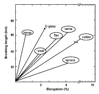
**Fig. 13-7** Breaking length versus elongation of some natural fibers. (Reprinted from Herrmann et al., 1998, Construction materials based upon biologically renewable resources—from components to finished parts, *Polymer Degradation and Stability* 59:251–261. With permission from Elsevier.)
