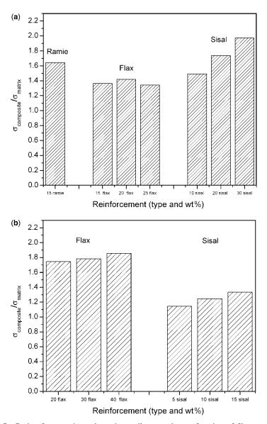
Fig. 11-8 Ratio of composite and matrix tensile strength as a function of fiber content for different fibers in (a) starch/polycaprolactone blends and (b) starch/cellulose derivative blends.
