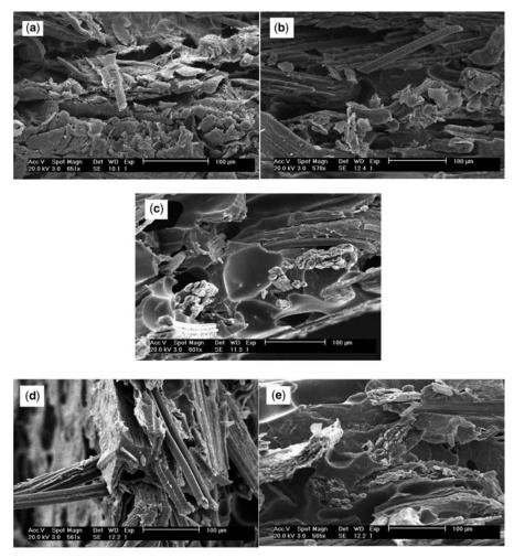
**Fig. 13-27** SEM images of the cross-section of (a) unmodified PHB composite, and composites with (b) 2.5% TDP, (c) 5% TDP, (d) 7.5% TDP, and (e) 10% TDP. (Reprinted from Wong et al., 2004, Interfacial improvements in poly(3-hydroxybutyrate)–flax fiber composites with hydrogen bonding additives, *Composites Science and Technology* 64(9):1321–1330. Reproduced with permission from Elsevier.)
