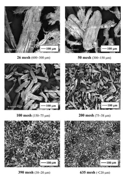
Fig. 12-3 SEM images of wood flour particles separated with sieves of different mesh sizes.
