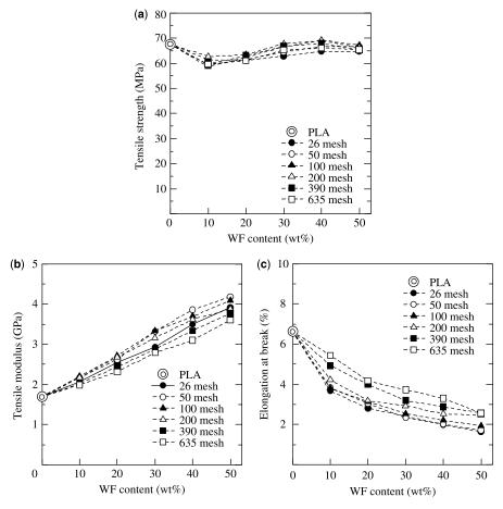
Fig. 12-4 Tensile properties of PLA/WF composites.
