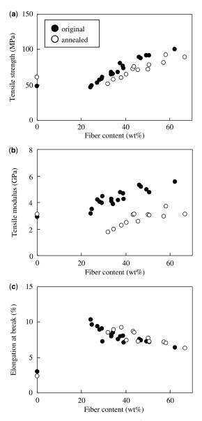
Fig. 12-8 Tensile properties of native and annealed PLA/lyocell composites as a function of fiber content.
