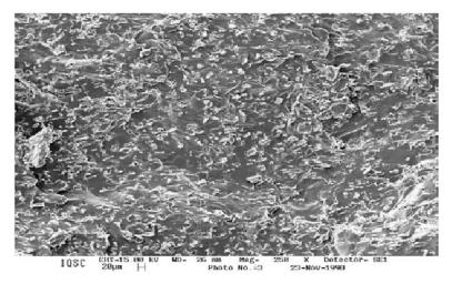
**Fig. 14-6** SEM image of a fragile fracture surface of 16% fiber-filled thermoplastic starch (30% glycerin) composite ( $250 \times$  magnification). (From Curvelo et al., 2001.)
