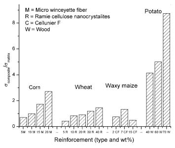
Fig. 11-7 Ratio of composite and matrix tensile strengths of different starches with degree of natural fiber incorporation.
