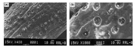
**Fig. 13-14** SEM images of coir fibers before (a) and after (b) alkali treatment. Scale bar given in 10  $\mu$ m. (Reprinted from Rout et al., 2001, Scanning electron microscopy study of chemically modified coir fibers, *Journal of Applied Polymer Science* 79, 1169–1177. Copyright 2001 John Wiley & Sons. Reprinted with permission of John Wiley & Sons, Inc.)
