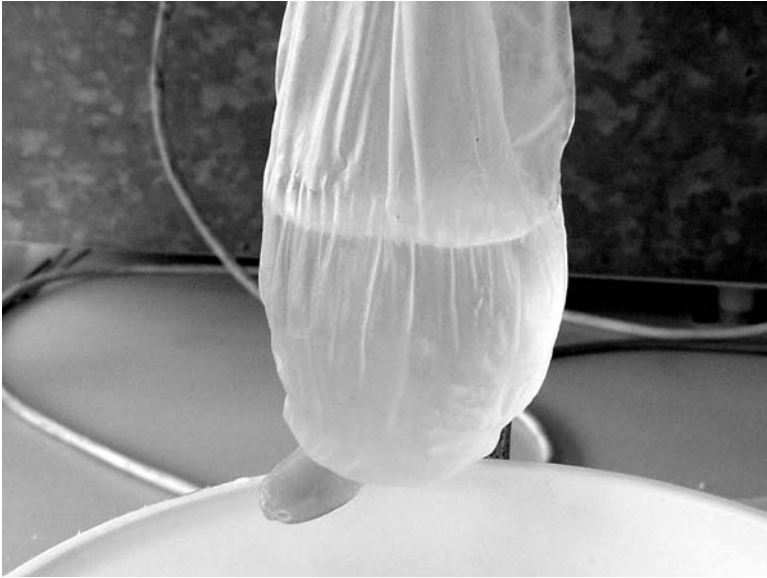
Fig. 15-2 A bag manufactured from a blown film of a TPS/5% montmorillonite nanocomposite plasticized with 30% glycerol/18% water. The bag was filled with water and stored for 20 days, showing excellent stability against cold water. (After Fischer et al., 2001.)
