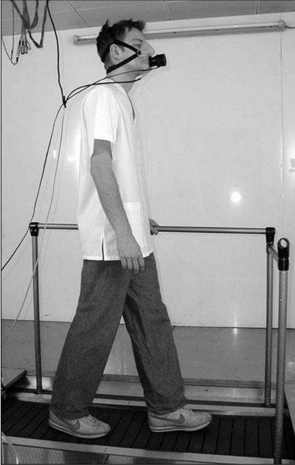
Fig. 3. Photo of a test person during wearer trials with tunics. The face mask is needed to determine the metabolic rate by analysing the exhaled air's oxygen and carbon dioxide contents.
