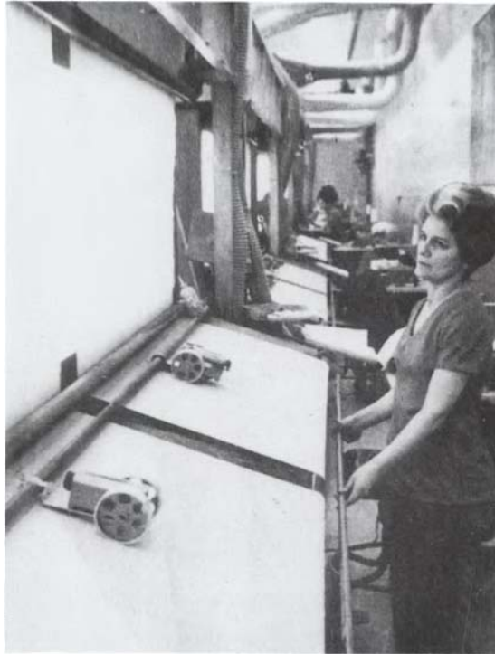
Figure 2-1. Perches used for inspection of fabric (Courtesy of Springs Mills).
