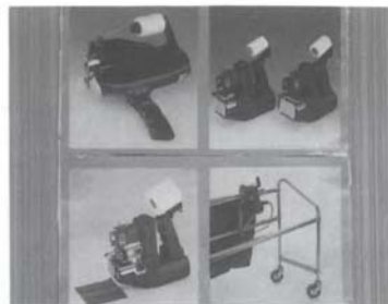
Figure 2-3(b). Overlocking machines for joining piece lengths of fabric (Courtesy of Metalplast, Italy).
