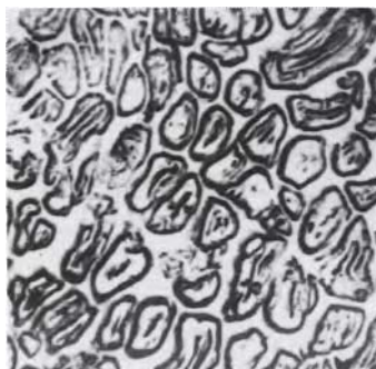
Figure 1-13. Cross-section of flax fibre (E.I.DuPont de Nemours & Co.).
