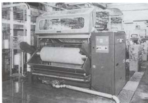
Figure 3-6. Universal Jigger for pre-treatment processes (Courtesy of Benninger AG, Uzwil).
