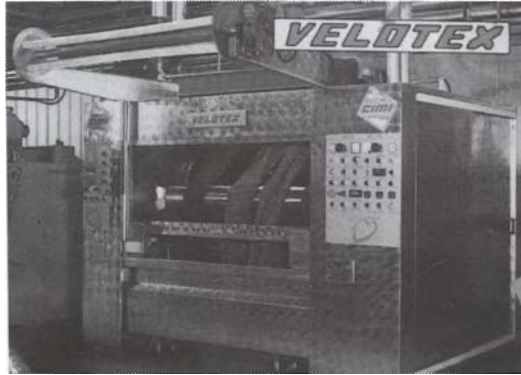
Figure 3-7. Machine for desizing and washing in the rope form [Courtesy Cimi S.R.L., (Biella), Italy].
