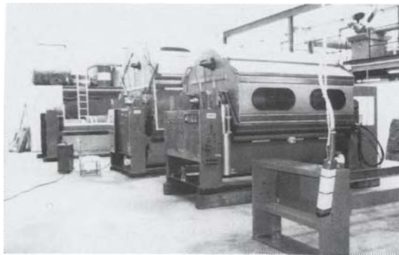
Figure 5-7. New generation of jiggers (Courtesy of Asyst S.L., Sabadell).
