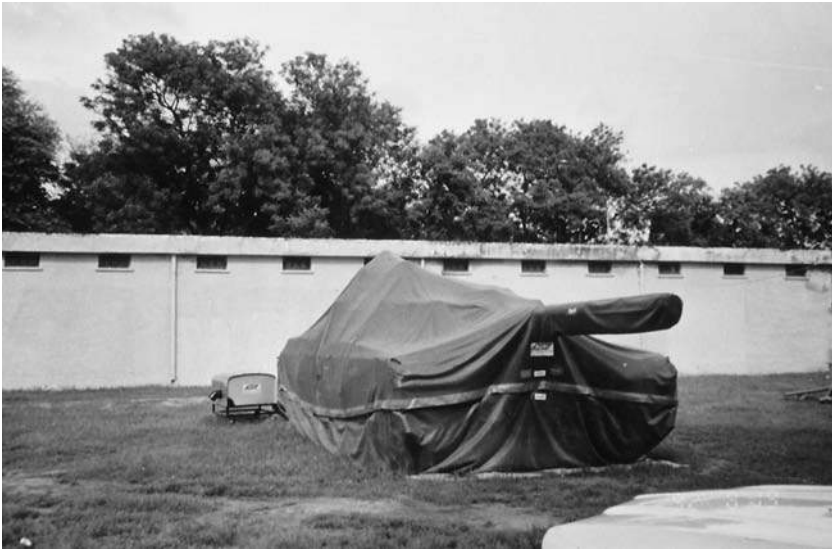
Figure 7.6 Flexible barrier system for protection of tank. Courtesy M/S Arctic India Sales, Delhi, India.
