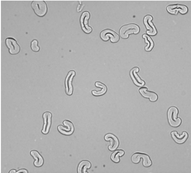
3.5 Cross-sections of cotton fibres embedded in methyl-butyl methacrylate resin showing cell wall and lumen (CSIRO Textile and Fibre Technology, Belmont, Australia).
