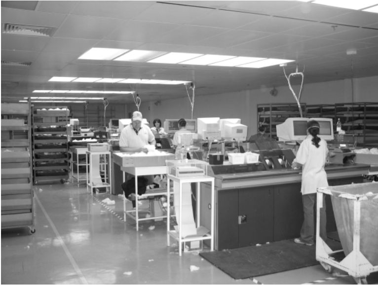
3.1 Modern high volume instrument (HVI) lines (photo courtesy of Australian Classing Services, Wee Waa, Australia).
