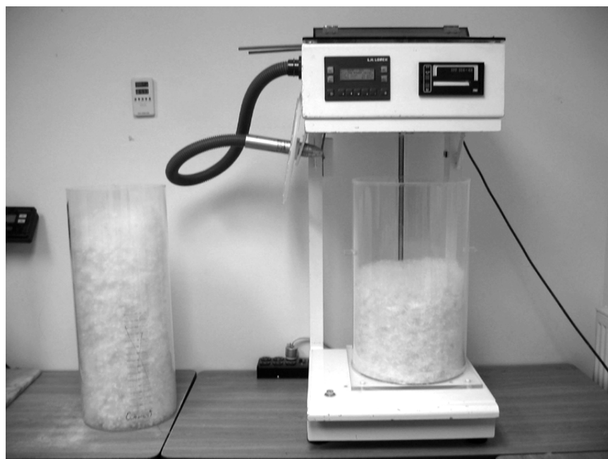
2.13 Filling power cylinders. Manual (left) and automated (right) (source: Peter Lieber).
