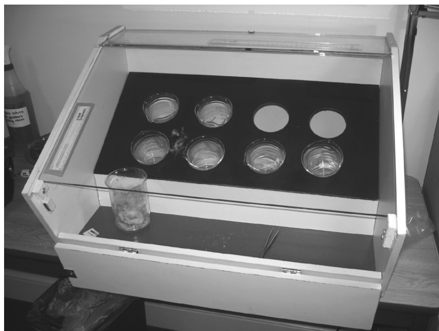
2.8 Separation cabinet (source: Peter Lieber).
