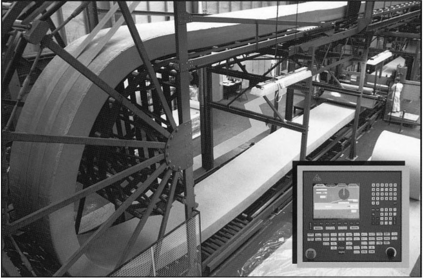
2.2 Production of sheet polyurethane foam for lamination to automotive seat cover fabric. The photograph shows Caligen Foam's 60m block slitting facility. Photograph supplied by Caligen Foam Ltd and reproduced with kind permission.
