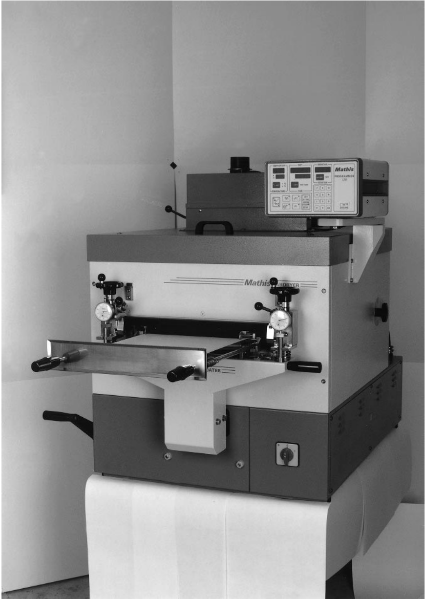
2.6 Mathis Type LTE-S laboratory coating machine with knife on air, knife on roller and knife on rubber blanket facilities. Air flow can be controlled above and below and can be set to any required temperature up to 200°C. Photograph supplied by Werner Mathis AG (R Jackson Wardle) and reproduced with kind permission.
