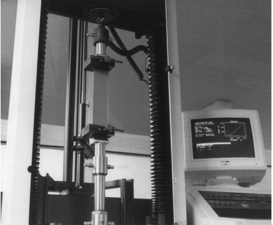
5.1 The universal tester is used not only for fabric tear and tensile strength determinations, but also extensively for coating and lamination adhesion testing (peel bond). The apparatus is also used for stretch and set testing which has become more important for moulding and automated manufacturing operations. Photograph supplied by Bobet Coated Fabric Company and reproduced with kind permission.
