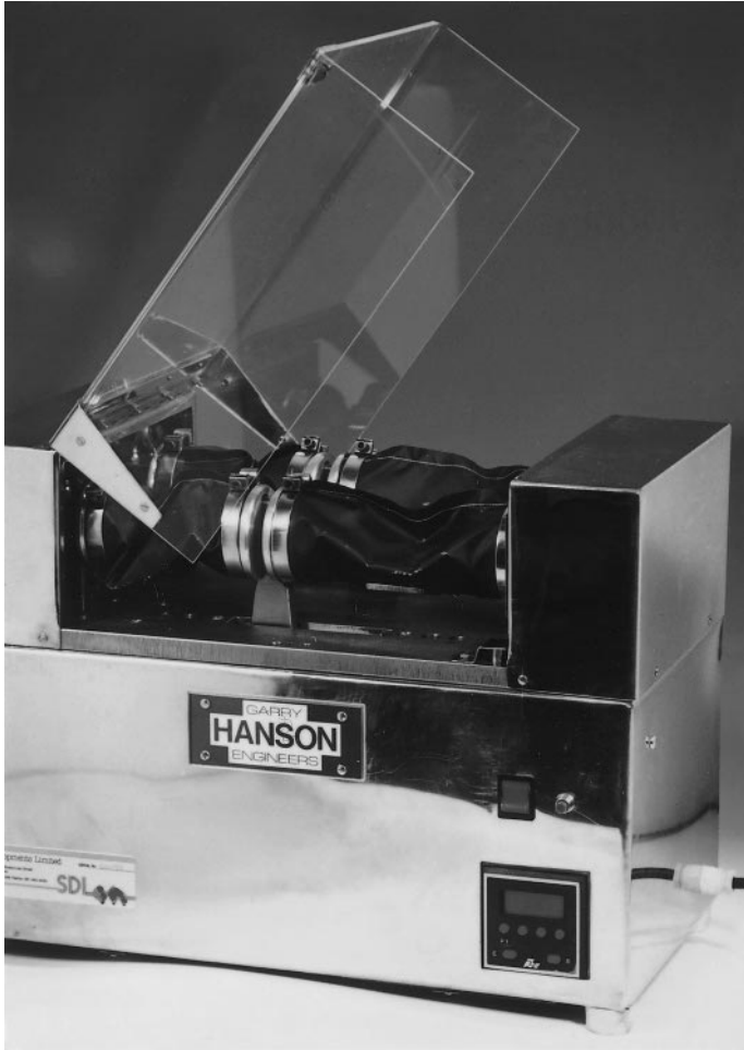
5.2 Crumple-flex testing is important to assess coating adhesion and quality under simulated wearing conditions. A tube of fabric is repeatedly flexed, stretched and compressed and twisted through 87°. Suitable for BS 3424, ISO 8096 and other tests. Photograph supplied by SDL International Ltd and reproduced with kind permission.
