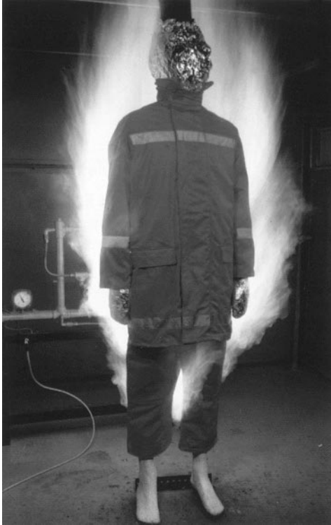
5.13 The BTTG Fire Technology Services RALPH manikin for full flame envelopment conditions. With each test, a burn injury prediction print-out is produced, providing information on first and second degree burn levels to allow users and garment manufacturers to evaluate performance under the most extreme of conditions. Fire-fighters' garments, FR coveralls for the off-shore oil industry and military clothing have been tested with this apparatus. Photograph supplied by BTTG and reproduced with kind permission.
