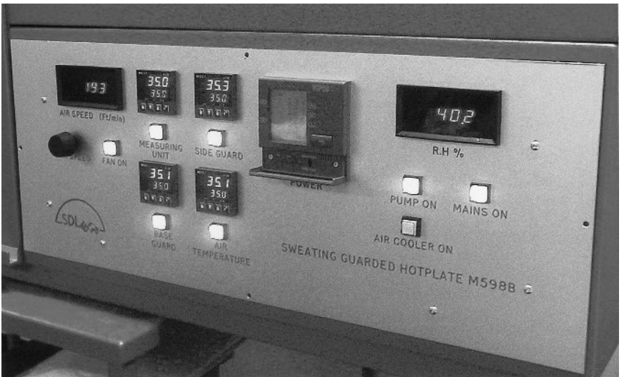
5.8 A commercial Sweating Guarded Hotplate test rig. Photograph supplied by SDL International and reproduced with kind permission.
