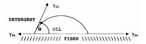
In order for the dynamic contact angle  $(\Theta_d)$  to change from zero to 180 degrees, the resultant (R) must be positive. R is positive when the quantity - (fiber/oil minus fiber/detergent interfacial tension) - is greater than the oil/detergent interfacial tension ( $\gamma_{F/O} - \gamma_{F/D} > \gamma_{O/D}$ ). It follows then that when R is greater than zero, the contact angle increases.
