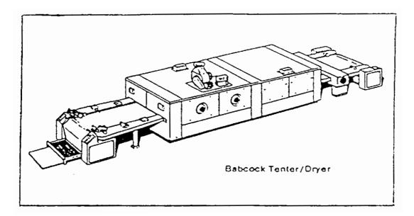
The heating section of a tenter frame also can be broken down into heating zones. The temperature in each zone can be independently set to profile any drying
