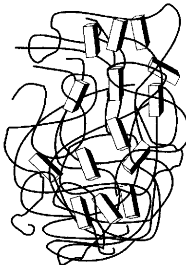
Figure 1.8 Simplistic 'bricks-in-mortar' two-phase representation of fibre fine structure (similar to that due to Nägeli, 1928).
