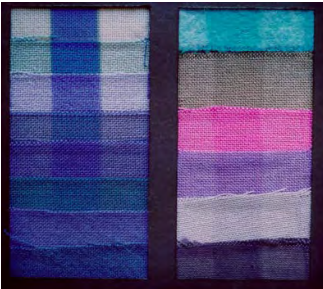
Plate 2 Standards for assessment of fading in light fastness testing
