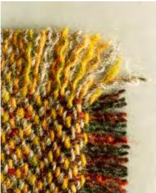
Plate 4 Harris tweed fabric, frayed out to show the differently coloured component fibres of each yarn
