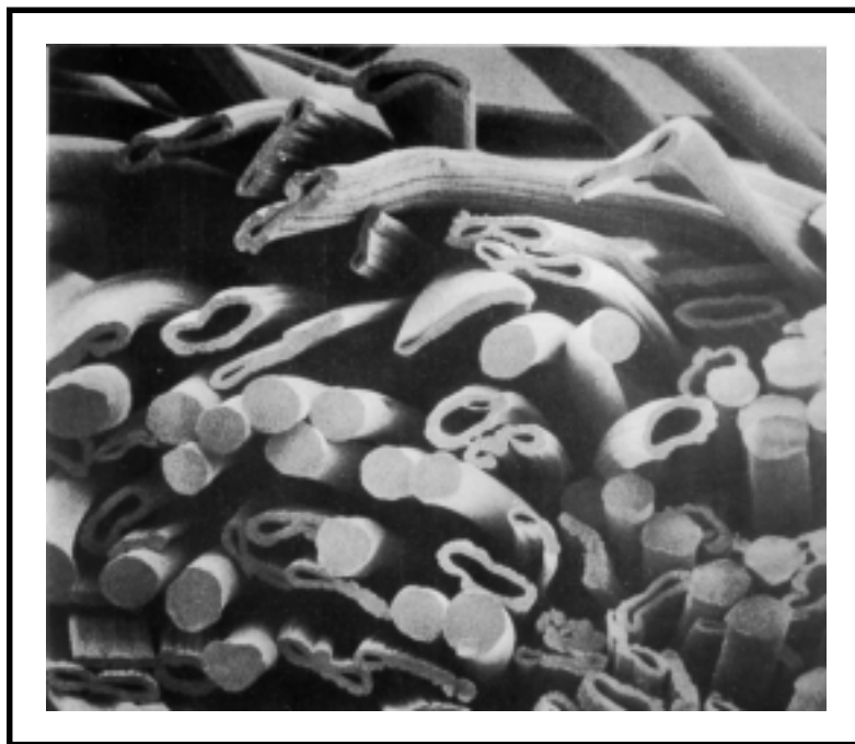
Figure 4.13 Cross-sections of polyester fibres (rod-shaped) and viscose fibres (hollow) in a fibre blend ( \times 750 )
