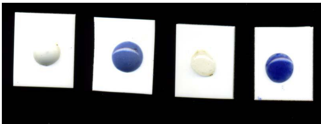
Figure 15. Stability of the \text{CoAl}_2\text{O}_4 nanoparticles in two commercial frits for high temperature.
