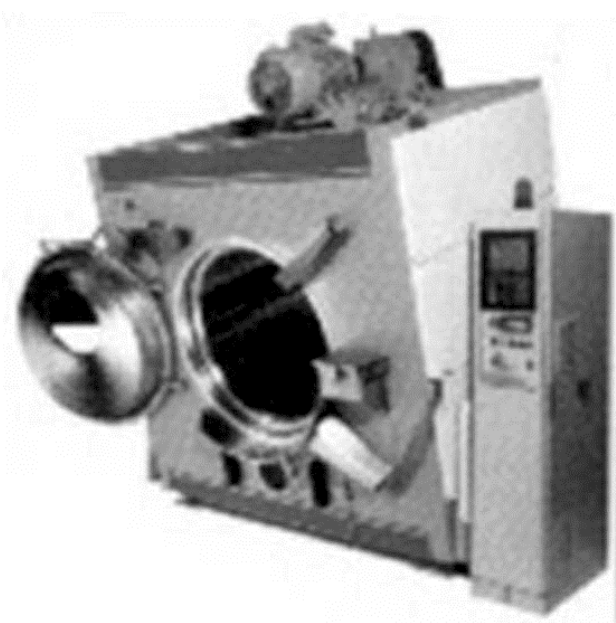
Picture 66 –Garment dyeing machine equipped with tilting device for unloading.
