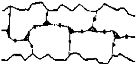
Picture 148 - Polyglucose chains cross-linked with cellulose reactants
