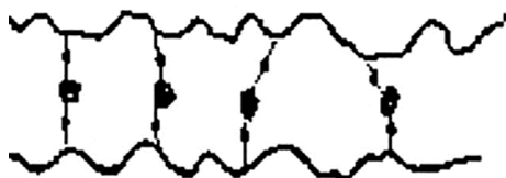
Picture 149 - Polyglucose chains cross-linked with thermosetting resins
