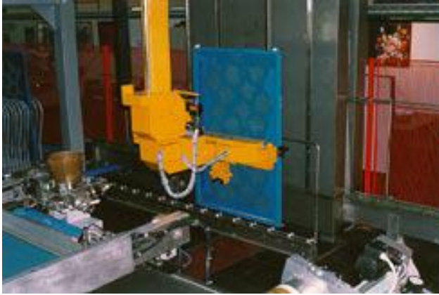
Figure 2.4 Robot lifting a flat screen from the rack prior to fitting it on the printing machine (Viero)
