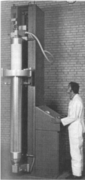
Figure 2.20 Semi-automatic rotary-screen coating machine (Stork Screens BV)
