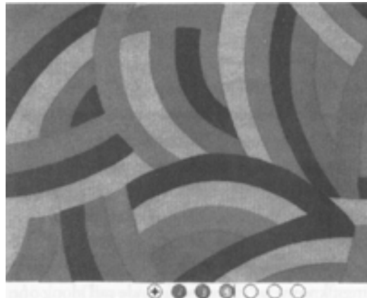
Figure 2.2 Pitch marks: the first screen prints all the circles and a cross in the first circle, the second screen prints colour in the second circle and a cross in the first circle, the third screen prints colour in the third circle and a cross in the first circle
