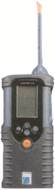
Figure 32.9. The Cyrano 320. The electronic nose may find uses in the food industry, animal husbandry, law enforcement, and medicine. [Courtesy of Cyrano Sciences.]
