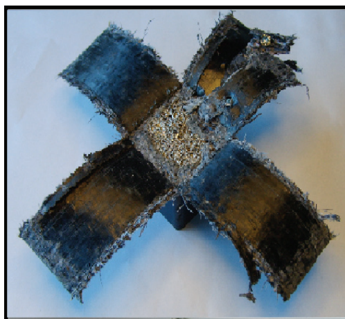
Fig. 16. Crush pattern of foam-filled composite crash box
