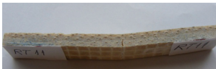
Fig. 36. Photo of the specimen surface made of E-glass EWR145 / fir wood flour / polyester Colpoly 7233 after immersion in water (5612 hours)
