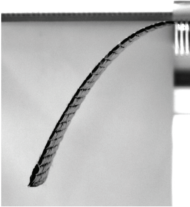
Fig. 10. Cantilever bending test
