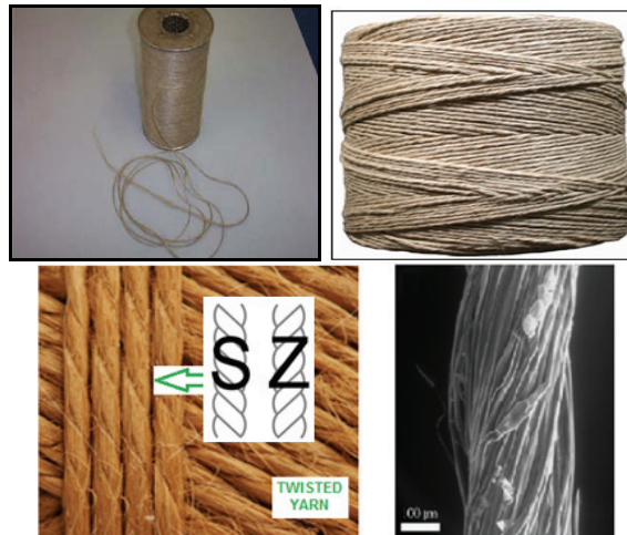
Fig. 9. Hemp twisted yarn and scanning electron microscope image of hemp twisted yarn
