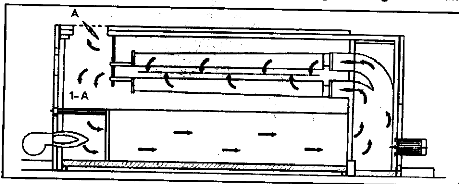
Air flows inside a stenter featuring a hot air convection drying system
