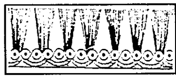
Tufted carpet with cut pile
