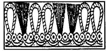
Tufted carpet with level-sheared pile
