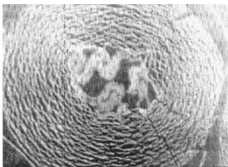
Fig. 2.12 Photomicrograph of a cross section of a single cotton fiber showing the development of growth rings. (From Ref. 40.)
