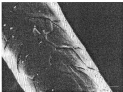
Fig. 2.22 Longitudinal view showing the scale structure of a mohair fiber. (From Ref. 62.)
