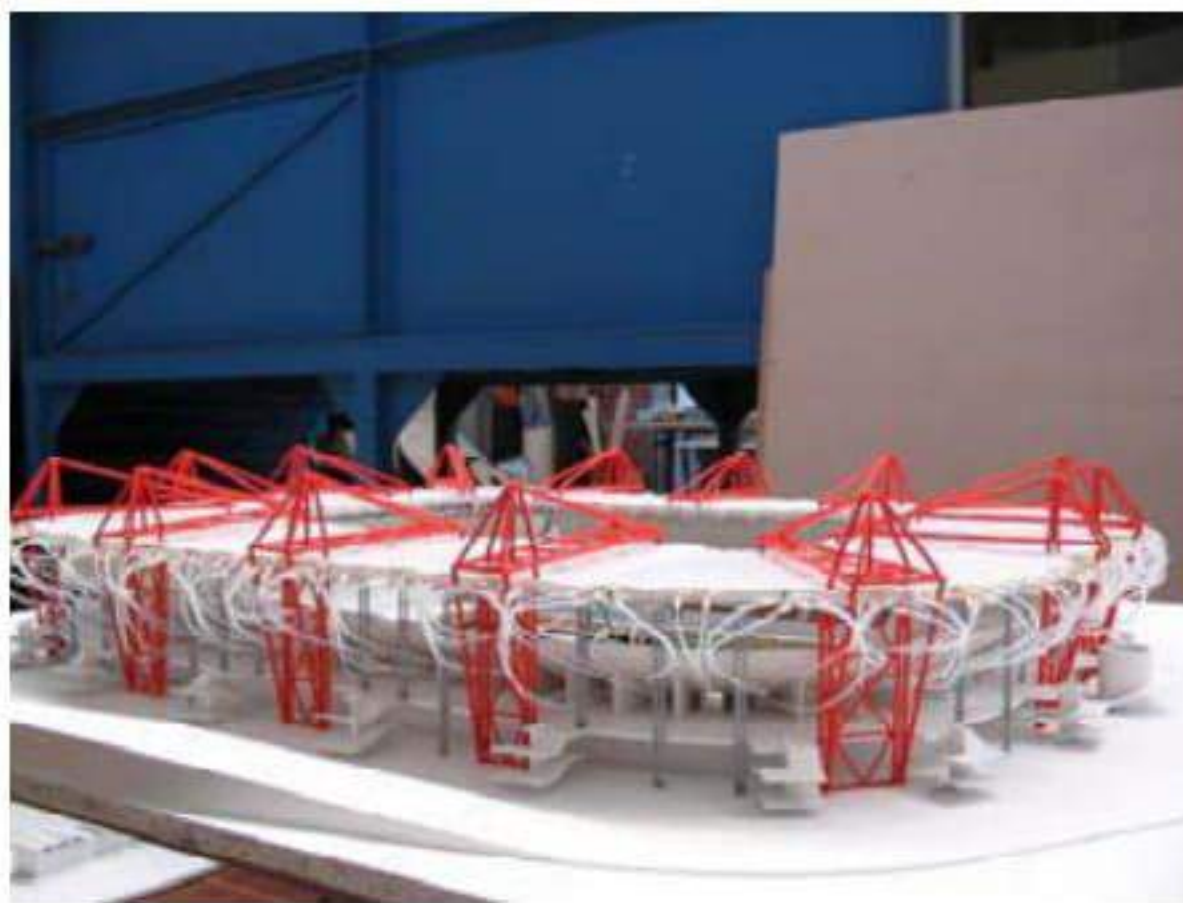
Fig. 12. Wind tunnel scale model
