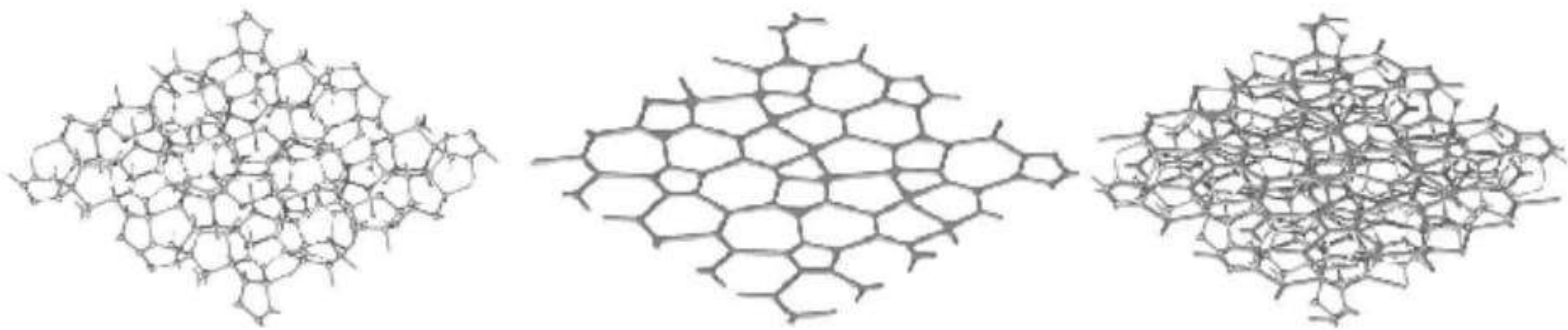
Figs. 50-52. From left to right: polyhedral space frame, flat face structure, combination of both. The face structure comprises a flat web of rectangular box sections either welded or bolted together on site. The face structure is added to the top and bottom of the space frame to complete the structure. [Ove Arup Plt ltd]
