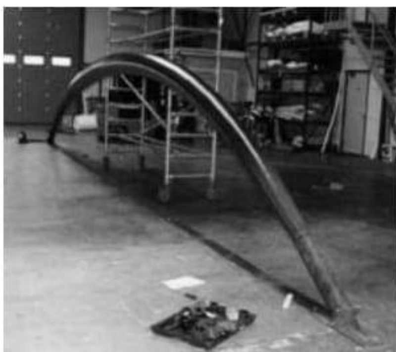
Fig. 9. Pneumatic mould supported by the auxiliary structure (Tentech/Buitink Zeilmakerij)
