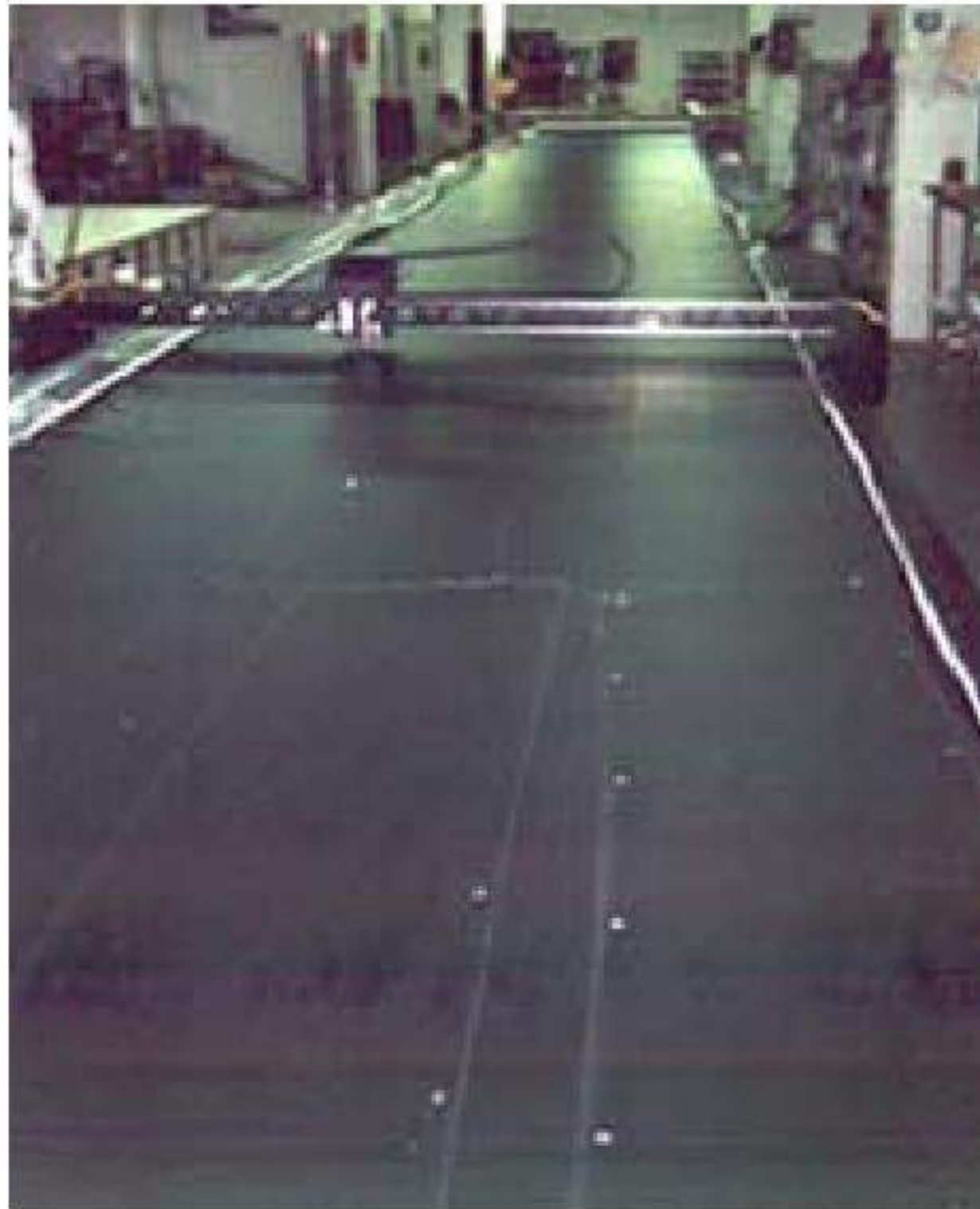
Fig. 7. Plotter system used to cut the membrane patches
