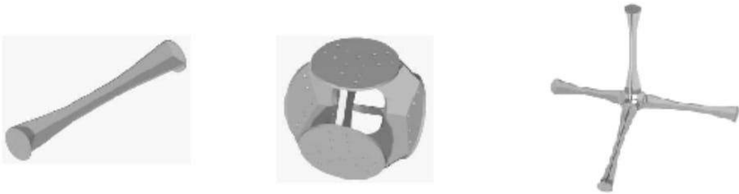
Figs. 47-49. The members are fabricated from three plates with circular end plates. The nodes are simple steel fabrications with circular plates for the end plates on the members and corresponding holes to receive the bolts. These two elements are simply bolted together to form an assembly. The assemblies are bolted together to form the space frame. [Ove Arup Pty Ltd]
