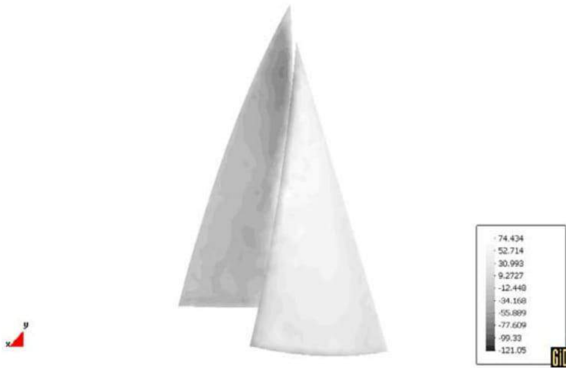
Fig. 4. Interaction of a genoa and a main sail - pressures at the end of the coupled analysis
