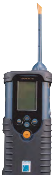
Figure 33.9 The Cyrano 320. The electronic nose may find uses in the food industry, animal husbandry, law enforcement, and medicine. [Courtesy of Cyrano Sciences.]
