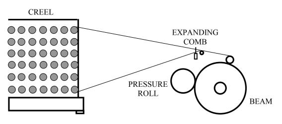
Fig. 18 – Beam warping machine.
