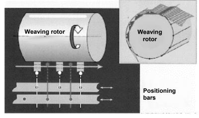
*Fig.* 104 – *The elements of the weaving rotor form, by plunging one after* the other into the warp yarn sheet, forming a sequence of sheds. The positioning bars select the threads to be raised through movements of only few millimetres.
