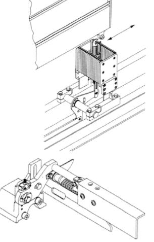
Fig. 98 – Quick beam change: this operation is facilitated by the quick insertion of the beam's end through grooved profile driven by an eccentric, while leaving the gear on board the weaving machine; the beam blocking is guaranteed by a quick gripping system
