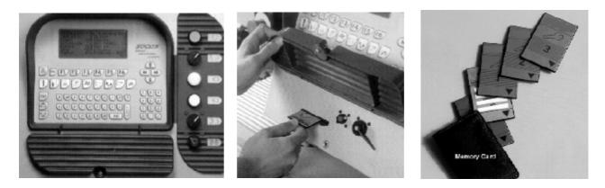
Fig. 91 – Board computer equipped with memory card
