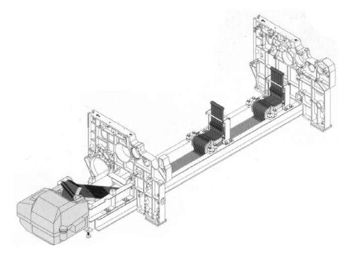
Fig. 74 – Skeleton of a weaving machine
