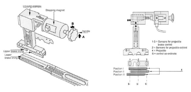
Fig. 52 – Brake adjustment
