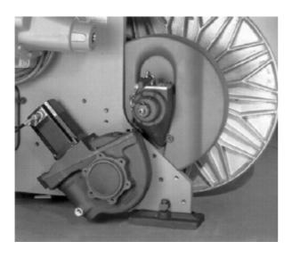
Fig. 78 – Servomotor for take-up motion drive
