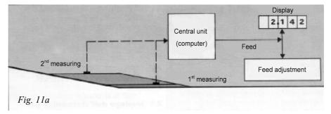
Soon after starting warping the first section, the actual thickness of the yarn wound on the dresser is measured and on basis of this value the extent of the feed is automatically corrected. To attain this result, the machine measures two times at the beginning of warping the dresser diameter (through an electronic precision micrometer), that is when the yarn layer reaches a thickness of 2
