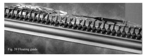
of special shape have been adopted; these pins, besides guiding the belts, keep them raised together with the pertaining rapiers, thus avoiding the sliding on the threads of the bottom shed during weft insertion.
