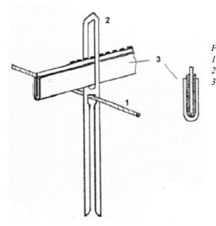
Fig. 110 – Electric warp stop motion: 1 – Warp thread 2 – Metallic drop wire 3 – Contact rail
