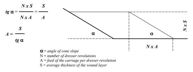
*Fig.* 10 – Correlation among feed, cone angle and average thickness of the wound thread layer.
