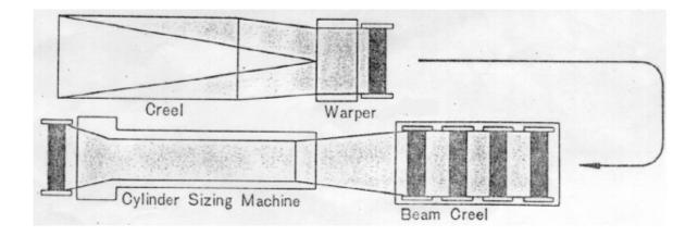
Fig. 26 – Conventional sizing: Creel: contains the cones Warper: warps the threads Beam creel: contains the beams Cylinder sizing machine: sizes the yarn
