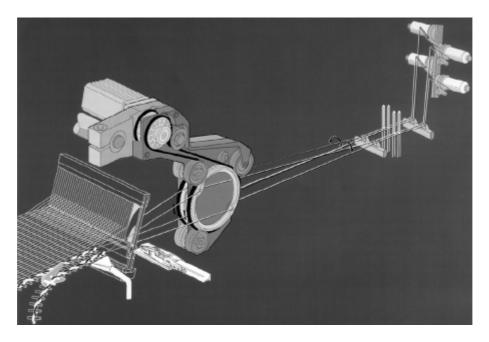
Fig. 116 – Double disk device for leno selvedges
