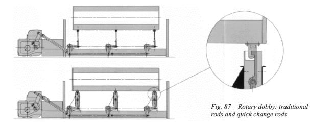
The insertion of the slider causes a 180° rotation of the plate which, thanks to the link, imparts a force on the lever controlling the rods of the heald frame, causing its passage from the initial position to the opposite position and consequently the raising of the heald frame.
