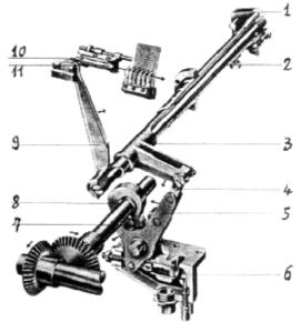
Fig. 48 - Projectile launching mechanism
