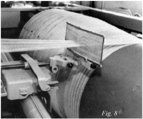
The carriage has a traverse motion and bears the *expanding or warping comb*, the *guide and metering roller* and the *levelling roller*.
