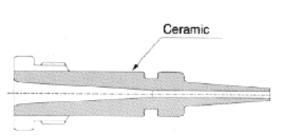
Fig. 62 – Cross-section of a ceramic nozzle
