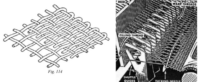
This system is generally used for light to middle weight fabrics, when weave and fabric density permit. There are also available tuck-in selvedge motions which are entirely controlled by pneumatic or mixed pneumatic and mechanical devices.
