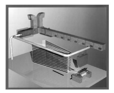
Fig. 123 – Conditioning in the warping room
