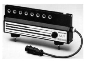
Fig. 108 – **Piezoelectric electronic weft stop motion** with integrated amplifier, which at its output emits two logic signals to indicate the broken weft or weft excess in the insertion.
