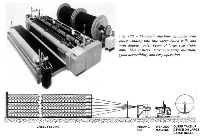
Fig. 101 – Weaving machine equipped with creel feeding and outer take-up device on large batch rolls (2000 mm diameter), used only for particular needs, like technical fabrics
