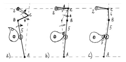
Fig. 49 – Loading of the torsion bar: a) torsion bar 2 in rest, knee-joint lever 4+5 in articulate position; b) loading phase; c) torsion bar in tension and knie-joint lever in stable position, before the launching control by roller 7.
