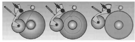
Fig. 20 – The increasing winding thickness of the yarn on the beam moves the pressure roller backwards.
