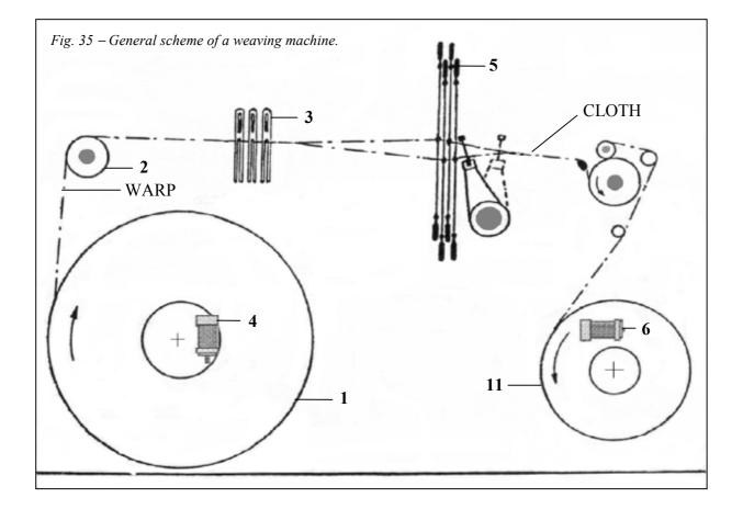
The warp threads wound on a beam (1) are bent on the back rest roller (2), support special drop wires (3), pass through the healds (5) and through the dents of the reed (8) fastened to the slay (7), along which the vehicle transporting the weft runs (9). The fabric produced is then drawn by a take-down roller(10) and wound on the cloth beam (11).
