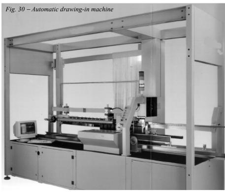
cotton twine which it inserts among the various elements of the warp stop motion, of the harness and of the reed according to the program set up on the computer and under its control and supervision.
