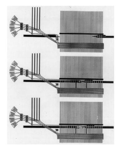
*Fig.* 36 – *Working principle of a rapier weaving machine.*
