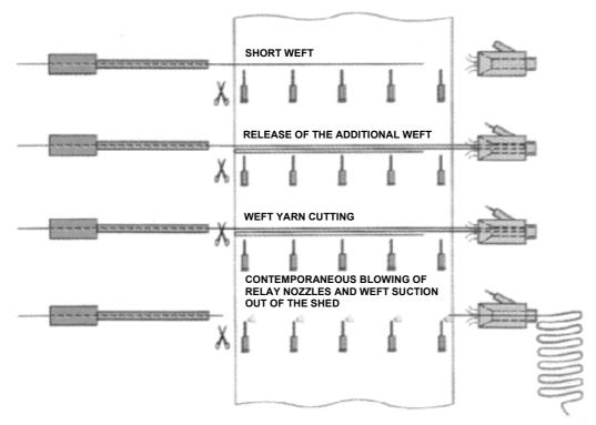
Fig. 59 – Automatic weft repair
