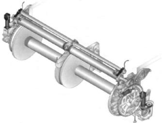
Fig. 80 - Example of double warp let-off motion for heavy weight fabrics or for fabrics with high warp yarn density (double width sizing machines and double capacity beam carriers would be required): the tension detecting system is independent on the two half-beams
