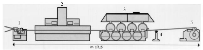
*Fig. 24 – Sizing machine: 1 – Size vat; 2 – Radio-frequency oven; 3 – Drum drying machine; 4 – Waxing device; 5 – Beaming.* 3
