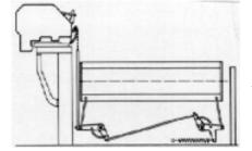
*Fig.* 84 – *Negative dobby (upper position for water-jet weaving machines)*
