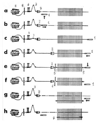
Fig. 50 – Insertion cycle of the projectile machine
