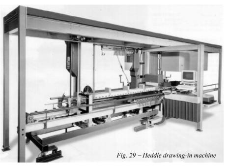
of long needle picks up in sequence the threads and inserts them with only one movement into the drop wires, the healds and the reed dents, which are selected each time and lined up to that purpose. The computer controls the different functions and supervises them electronically, ensuring the exact execution of the operation and interrupting it in case of defects.
