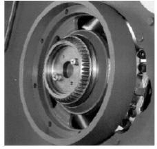
Fig. 21 Conical toothing.
