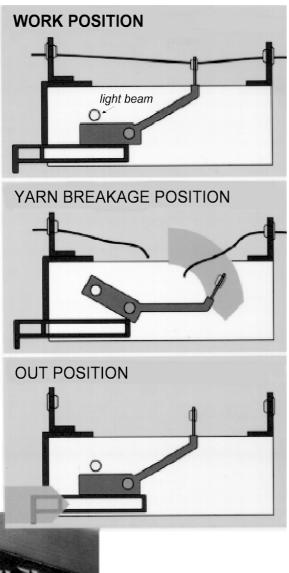
*Fig.* 5*a* – *During warping the thread supports the drop pin and the light beam is not interrupted.*
