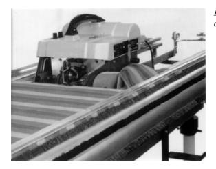
*Fig. 34 – Harness loading in the weaving machine.*
