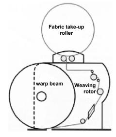
*Fig. 103 – Structure of the multiphase* multilinear weaving machine
