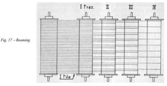
The way in which threads are assembled during this second phase shows that the number of the beams should be preferably an integer number.
