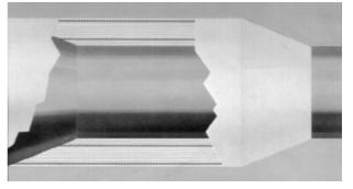
Fig. 11b – Correct winding up of the warp on the drum. Warping with same number of revolutions produces identical thickness of thread layers.
