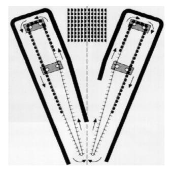
Fig. 3 – Swivel frame creel: this type of creel was designed as a variation of the mobile creel to enable the creeling up of bobbins which, owing to their heavy weight (5 to 25 kg), cannot be pinned on trolleys. Each bobbin holder is double-sided: the threads are unwound from one side, while a new series of bobbins is creeled up on the other side.
