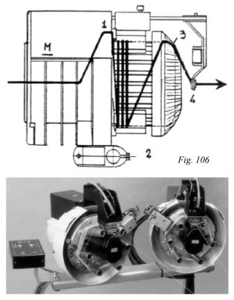
Fig. 107 – Pre-feeders for water jet machine with microprocessor controlled weft selection
