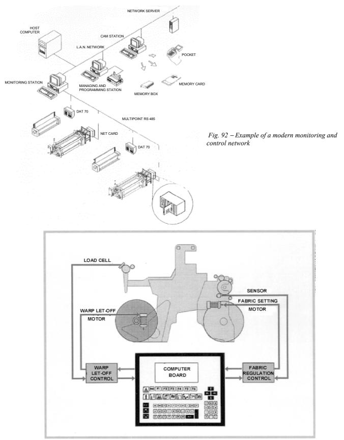
*Fig.* 93 – *Electronic detecting and control system on thread tension. Setting and modification of tension and weft density directly via board computer*
