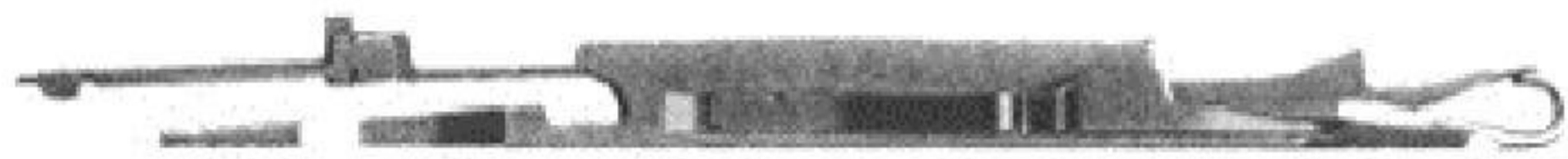
Picture 69 – A compound needle of a coarse-gauge flat knitting machine
