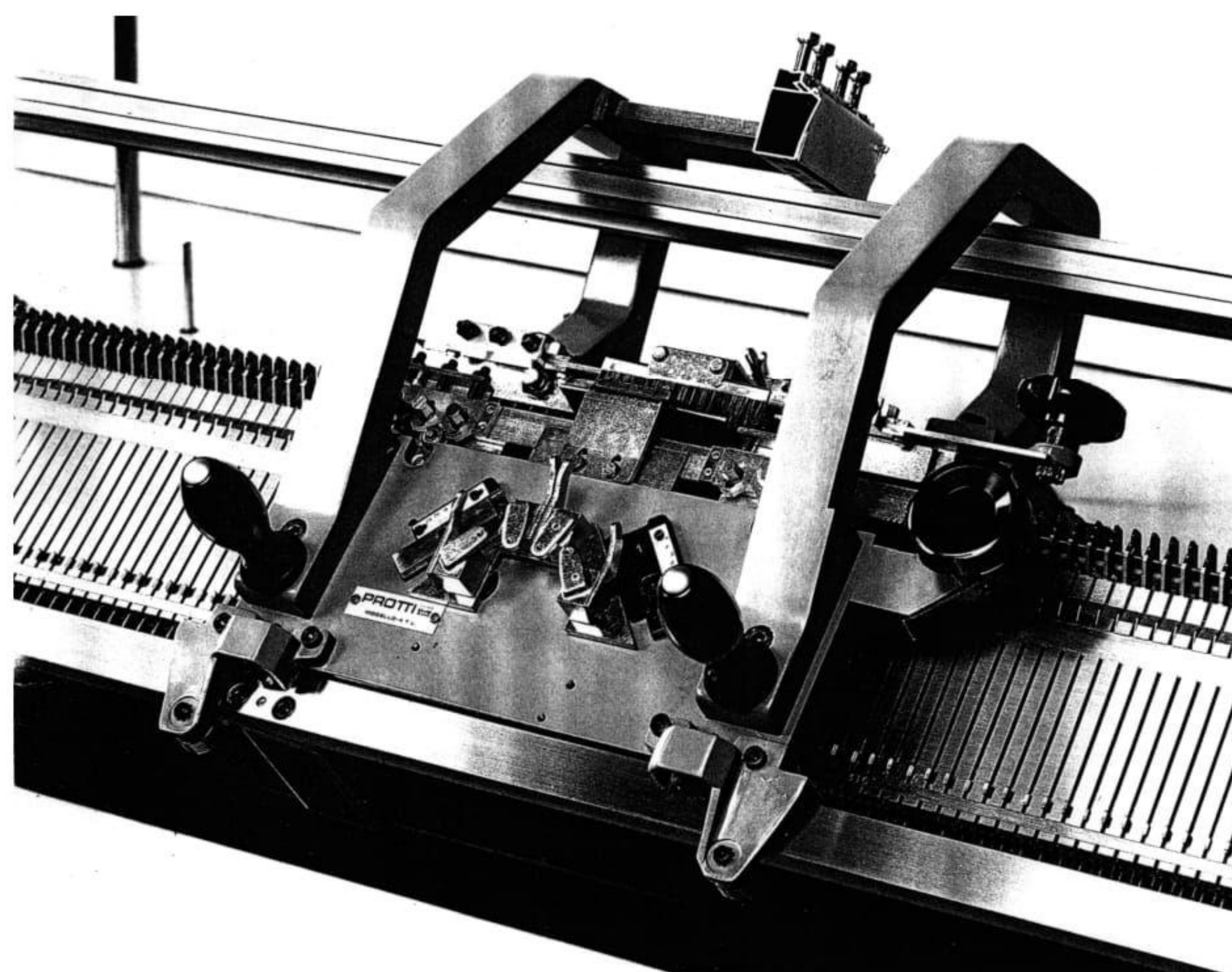
Picture 23 - Needle-bed and carriage of a manual flat knitting machine
