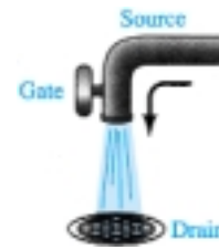
Figure 5.3 Water analogy for the JFET control mechanism.
