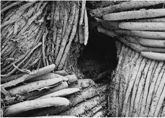
13.15 Scanning electron micrograph showing mechanical damage from abrasive particles.
