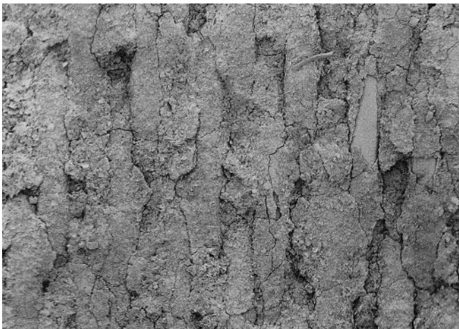
13.13 Scanning electron micrograph showing used fabric before cleaning.
