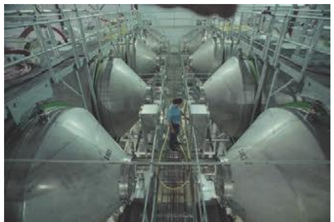
FIGURE 1 Industrial-scale fermentations to produce biofuel and other products are typically carried out in tanks that hold thousands of liters of medium.
