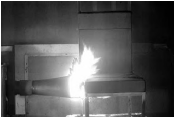
12.19 FAR 25.853(a) Appendix F Part II kerosene burner test for aircraft seating.
