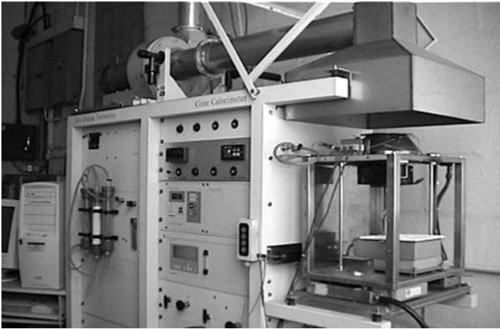
12.11 Cone calorimeter apparatus.
