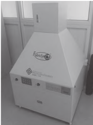
6.6 Two-dimensional image capturing system.
