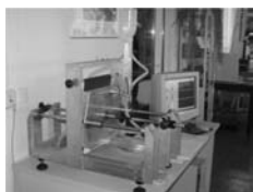
10.4 General view of apparatus for testing thermoregulation properties of fabrics containing PCMs (Bendkowska et al. , 2005).
