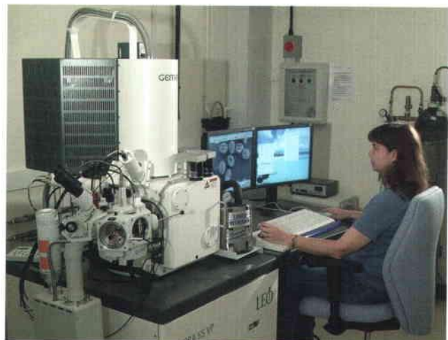
Figure 9-49 The scanning electron microscope. In a SEM, the specimen is scanned by a beam of electrons brought to a focus on the specimen by the electromagnetic coils that act as lenses. The detector measures the quantity of electrons scattered or emitted as the beam bombards each successive point on the surface of the specimen and controls the intensity of successive points in an image built up on a video screen. The SEM creates striking images of three-dimensional objects with great depth of focus and a resolution between 3 nm and 20 nm depending on the instrument. (Photograph courtesy of Andrew Davies.)
