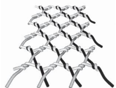
1.32 Geometric approach to textile modelling for a range of textiles, showing vectorial description of yarn paths (left) and resulting textile models (right).
