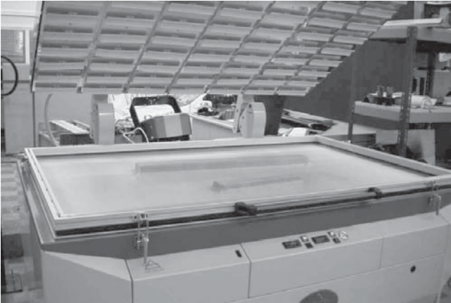
11.16 Heated vacuum performing facility used to form textiles coated with heat activated adhesive binders.
