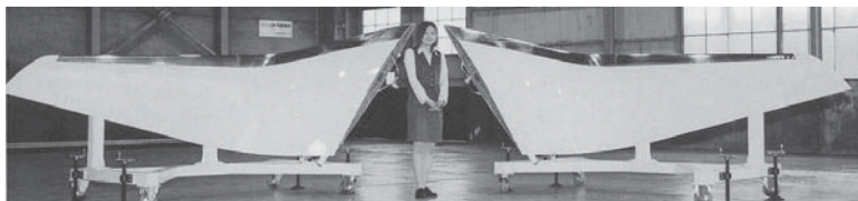
11.4 Boeing 737-300 winglet programme for Aviation Partners Boeing. Supplied by Kawasaki Heavy Industries (Japan); manufactured using KMS6115 style, Tenax HTS 12K fabric prepreg.
