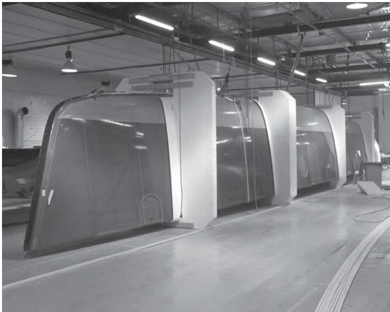
5.2 A large boat hull being manufactured using the SPRINT™ process. Figure reproduced by kind permission of SP Systems Ltd.
